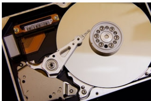
A read-write head of a hard drive
