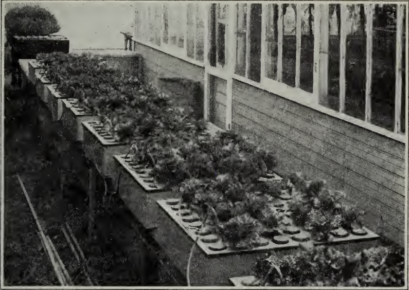
Fig. 2.—The use of the water-culture technique for studying the nutritional responses of lettuce plants under controlled conditions. The individual plants are supported in corks which are placed in holes drilled in the metal covers. The glass and rubber tubes carry air under pressure, which is bubbled through the nutrient solution in the tanks.
