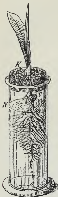
Fig. 1. — Water-culture installation employed by the plant physiologist Sachs in the middle of the last century. (Reproduced from Sachs, Lectures on the Physiology of Plants , Clarendon Press, 1887.)
