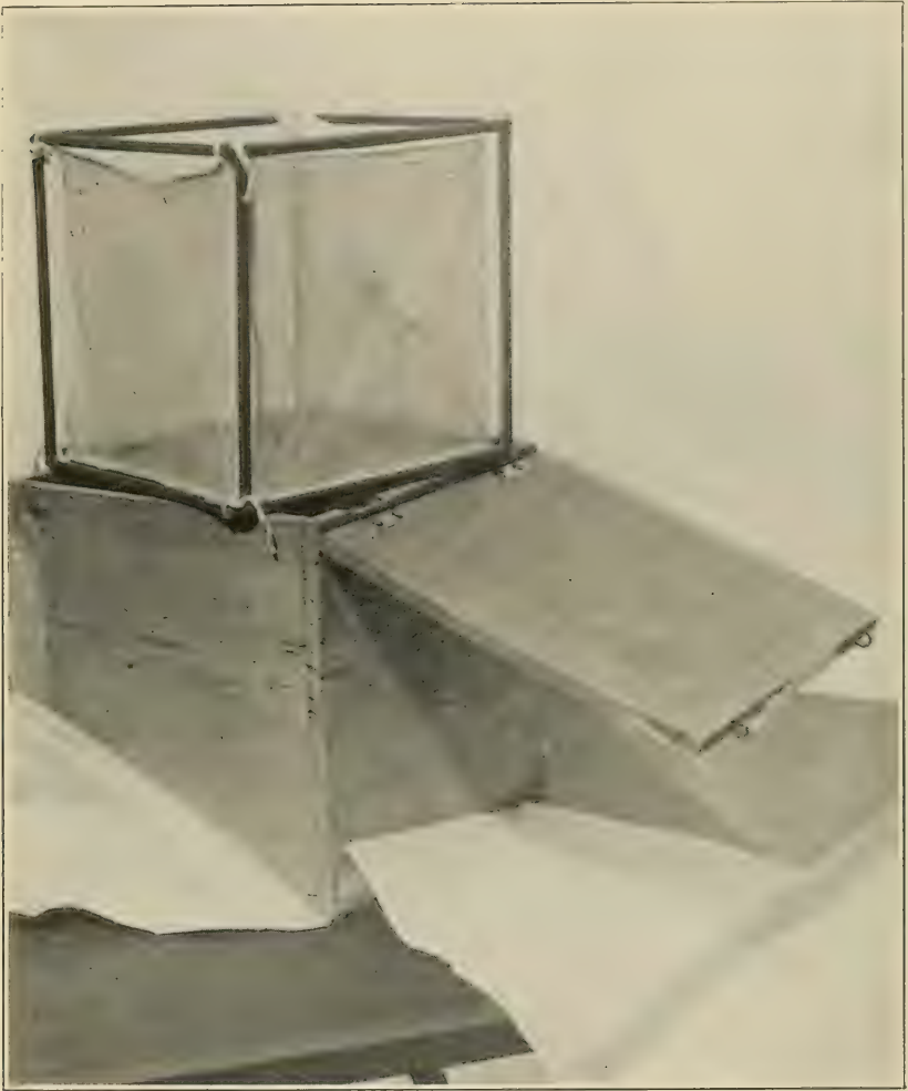
Figure 1. —Shipping box and cage for anopheles adults (modeled after Barraud's box used in India).
